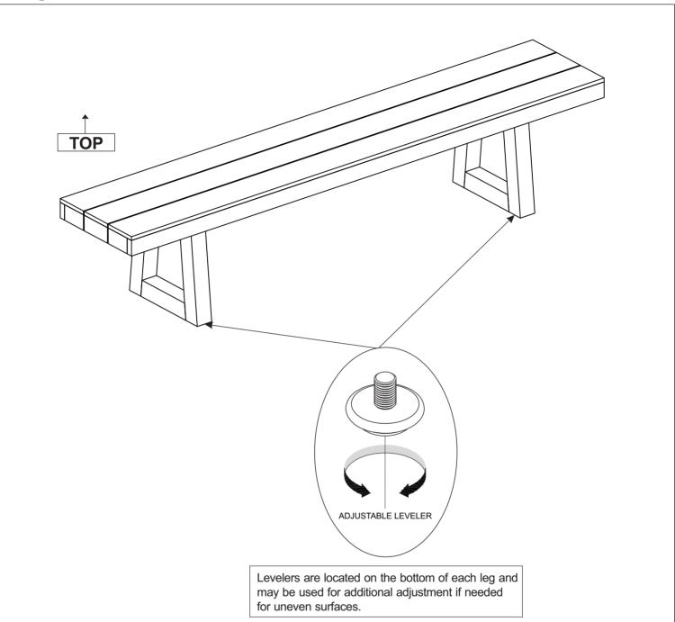
Using a second person to assist you, carefully turn the Bench right side up. Assembly is now complete and the product is ready for use. Adjustable levelers are located on the bottom of each leg and may be adjusted by turning outwards, counter-clockwise to help account for uneven surfaces.
