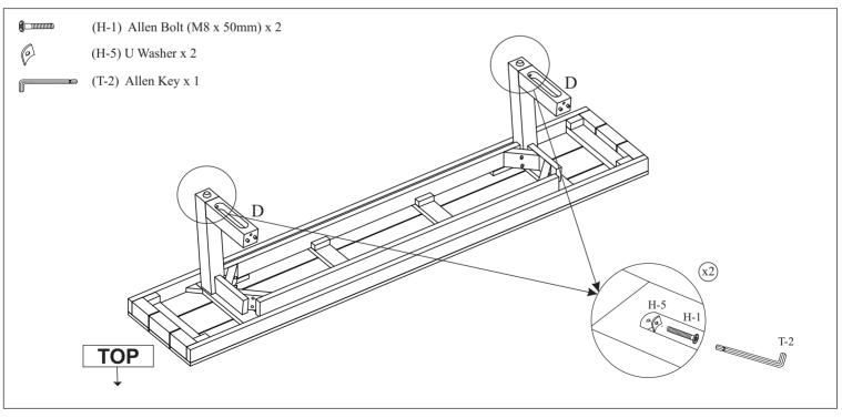
Insert the dowels in Leg Support Stretcher (D) into the receiving holes in Right Leg (B). Secure the connection with a Bolt (H-1) and a U-Washer (H-5) using the provided Allen Key (T-2), stacking the hardware in the order as shown. **Secure but DO NOT YET FULLY TIGHTEN.** Repeat the process for Left Leg (C).
