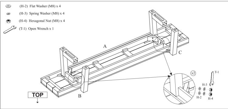
Insert the dowels in Leg Support Stretcher (D) into the receiving holes in remaining Right and Left Legs (B and C) as shown. At the same time, insert the hanger bolts in Right and Left (B and C) through the pre-drilled corner holes on Bench Top (A). Secure Right and Left Legs (B and C) with Flat Washers (H-2), Spring Washers (H-3) and Hexagonal Nuts (H-4) using the provided Open Wrench (T-1), stacking the hardware in the order as shown. **Secure but DO NOT YET FULLY TIGHTEN.**
