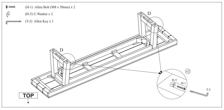
Secure both Leg Support Stretchers (D) to corresponding Right Leg (B) and Left Leg (C) using Bolts (H-1) and U-Washers (H-5) using provided Allen Key (T-2), stacking the hardware in the order as shown. Fully tighten ALL and Bolts (H-1) and Hexagonal Nuts (H-4) from this and all previous steps. DO NOT OVER TIGHTEN.
