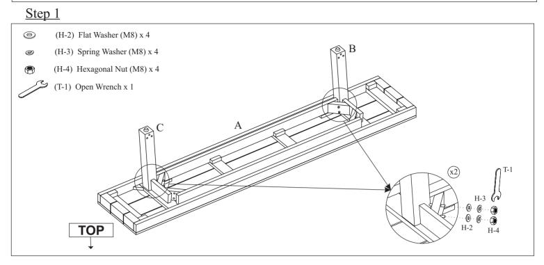
Using a second person to assist you, lay Bench Top (A) upside down onto a padded, non-marring surface. Position Left Leg (B), Right Leg (C) as shown, inserting the hanger bolts through the pre-drilled corner holes on Bench Top (A). Secure Left Leg (B), Right Leg (C) to the corner blocks with Flat Washers (H-2), Spring Washers (H-3) and Hexagonal Nuts (H-4) using the provided Open Wrench (T-1), stacking the hardware in the order as shown. **Secure but DO NOT YET FULLY TIGHTEN**.
